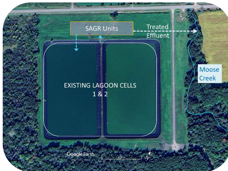
Figure 10-6: Process Flow Diagram for SAGR Retrofit
